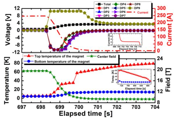
**Fig. 7.** Quench protection behavior of the insert with MI winding and PS voltage limitation techniques at  $I_{op} = 247$  A under  $B_{ext} = 9$  T at 4.2 K.
