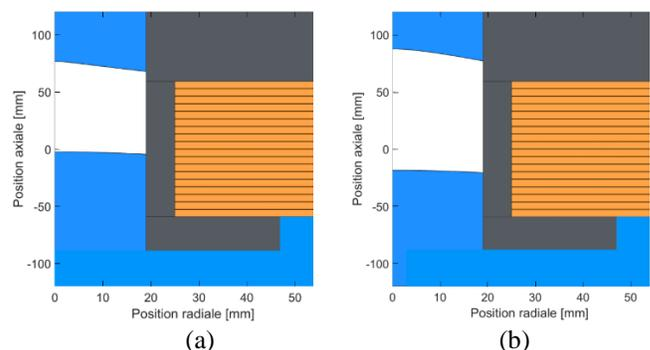
**Fig. 5.** Simulation results of trapped bubble position under same condition in Fig. 4:  $B_{\text{ext}} = 10$  T (a); and 18 T (b) at 4.2 K.
