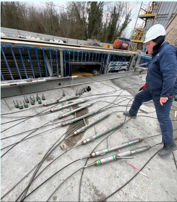
The downhole receiver toolstring is fully checked and re-tested on surface.
