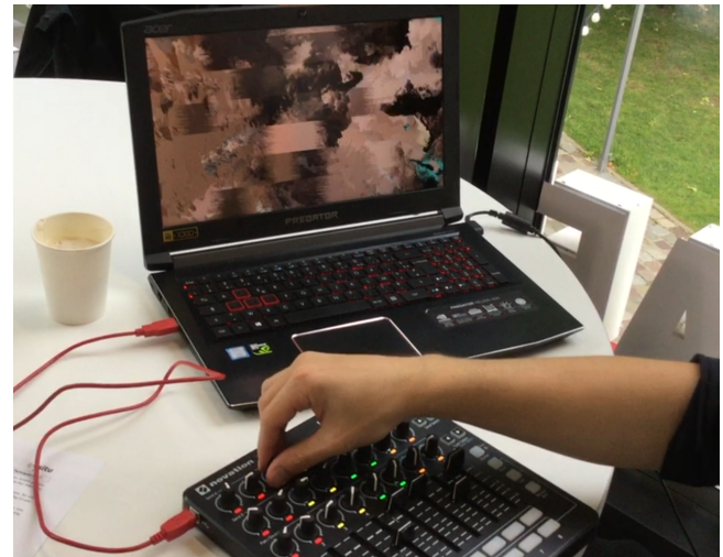
Figure 1: MIDI-controlled interactive glitch-art system (P1)
