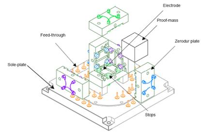
**Fig. 4.** Mechanical core of the  $\mu$ star accelerometer
