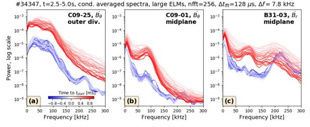
**Figure 7.** Conditionally averaged spectra during the phase dominated by type-I ELMs (2.0 < t < 5.0 s), for three magnetic coils: (*a*) C09–25 (outer divertor,  $\vec{B}_{\theta}$ ); (*b*) C09–01 (mid-plane,  $\vec{B}_{\theta}$ ); (*c*) B31–03 (mid-plane,  $\vec{B}_r$ ). Unlike B31–03 and C09–01, the average shape of the C09–25 spectra remains qualitatively similar during an ELM.
