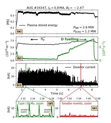
**Figure 2.** Time traces of (*a*) the plasma stored energy, (*b*) the line-averaged density  $\bar{n}_e$  measured by a central interferometry chord, and the Deuterium fuelling rate, (*c*) current on the inner divertor used as an ELM monitor (*d*) and (*e*): zooms in time windows of 80 ms showing the inner divertor current during phases with large and small ELMs.
