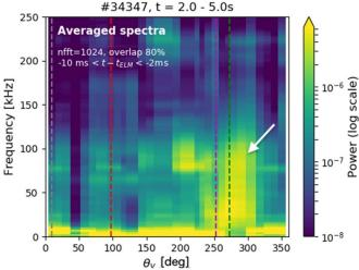
**Figure 6.** Conditionally averaged spectra of the magnetics signal from the poloidal array, during the phase with type-I ELMs #34347, 2 < t < 5 s, for  $-10 < \Delta t_{EL} < -2$  ms. The arrow indicates the region of broadband inter-ELM activity poloidally located close to the outer divertor.
