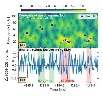
**Figure 8.** (*a*) Spectrogram of the signal from coil C09–25 (outer divertor), calculated using a short time window of 256 points ( $\Delta t = 128 \,\mu$ s), with a 90% overlap. Dominant frequencies evaluated using a sinusoidal fit in short time-windows are represented by the blue squares. (*b*) Corresponding signal, showing short-lived oscillations dominated by different frequencies in the range 15–80 kHz.
