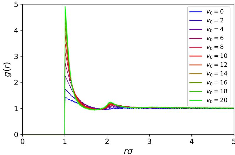
**Figure 4.** Radial distribution function  $g(r)$  of an active Brownian hard-disk system at packing fraction  $\eta = 0.2$ , for self-propulsion velocities  $v_0 \in [0, 20]$  (in steps of two, from bottom to top at  $r = 1^+$ ).
