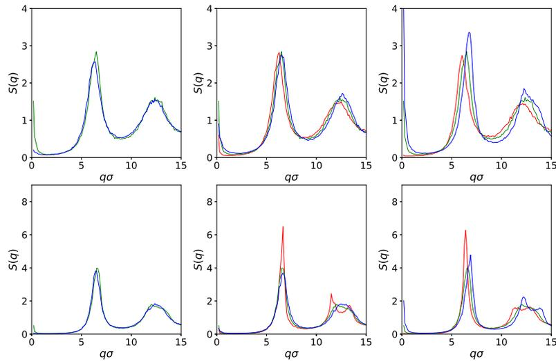
**Figure 8.** Static structure factor of active hard-disks fluid at packing fraction  $\eta = 0.6$  (top row) respectively  $\eta = 0.7$  (bottom row) with different rotational diffusion coefficients  $D_r = 0.1, 1,$  and  $10$  (red, green, blue), at constant  $Pe_t = 10$  (left), constant  $Pe = 100$  (middle), and constant  $Pe_r^{-1} = 10$  (right). Results are omitted for the state point ( $Pe_t = 10, D_r = 0.1$ ), where the system is already phase separated.
