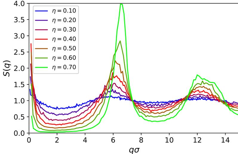
**Figure 2.** Static structure factor  $S(q)$  of active Brownian hard disks with self-propulsion velocity  $v_0 = 10 D_t/\sigma$  and rotational diffusion coefficient  $D_r = 1 D_t/\sigma^2$ , for packing fractions  $\eta = 0.1, 0.2, 0.3, 0.4, 0.5, 0.6,$  and  $0.7$ .
