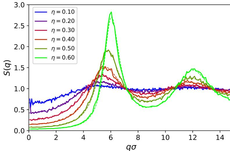
**Figure 1.** Static structure factor  $S(q)$  of passive hard-disk systems with packing fractions  $\eta = 0.1, 0.2, 0.3, 0.4, 0.5,$  and  $0.6$  (top to bottom around  $q\sigma = 2$ ). Solid lines: results from ED-BD simulations. Dashed lines represent the Baus-Colot expression for  $S(q)$ .
