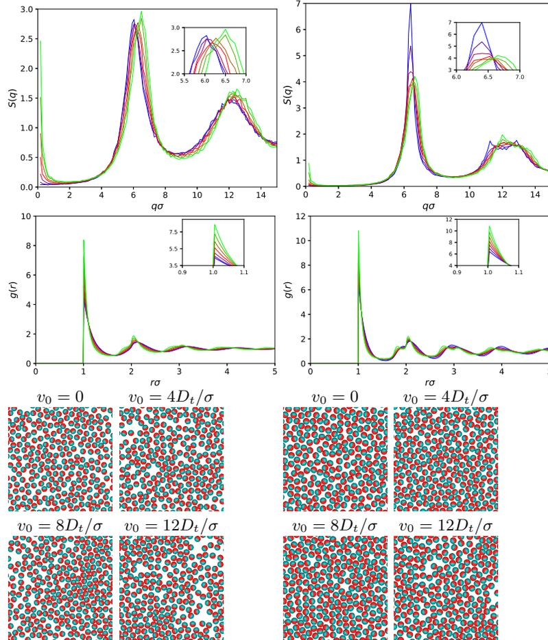
**Figure 5.** High-density fluid regime: static structure factor  $S(q)$  (top row), radial distribution function  $g(r)$  (middle row), and snapshots (bottom row) of active hard disks with packing fraction  $\eta = 0.6$  (left column) respectively  $\eta = 0.7$  (right column). Different curves correspond to different self-propulsion speeds  $v_0 = 0, 2, 4, 6, 8, 10, 12$  (from blue to green; curves ordered by increasing first-peak position in  $S(q)$  from left to right).
