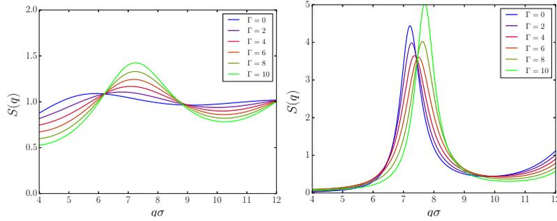
**Figure 6.** Static structure factor  $S(q)$  of a three-dimensional square-well system with short-ranged attraction (range  $0.1\sigma$ ), as a function of attraction strength ( $\Gamma = 0, 2, 4, 6, 8$ , and  $10$ ; blue to green), for moderate density (left panel; three-dimensional packing fraction  $\varphi = 0.1$ ) and for high density (right panel;  $\varphi = 0.55$ ).
