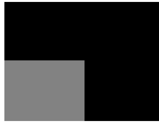
Figure 9: Phase screen used to generate the phase differences between sections of the wavefront. The lower left corner (shown in grey) had its grey levels vary between 0 and 250, while the rest of the phase screen was set to a grey level of 0.
