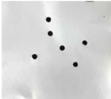
Figure 2: Non-redundant mask used for the SAWFS experiment. Thin sheet of aluminium with 1.5 mm holes. Unused holes were blocked as needed.
