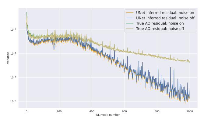
Figure 5: Variance (log) between KL modal weights of the inferred wavefront estimates and simulated ground truth
