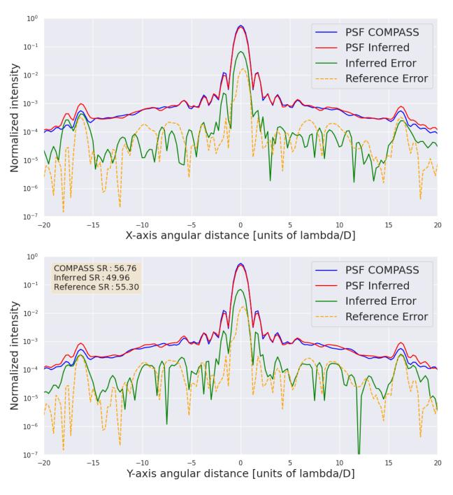
Figure 7: Long Exposure PSF-R analysis with RON of 1 and photon noise - x and y splits of the long exposure PSF for magnitude 12 guide star, near the limit of closed loop linear control stability. - 396 photons per sub-aperture,  $r_0=0.10\mathrm{m}$
