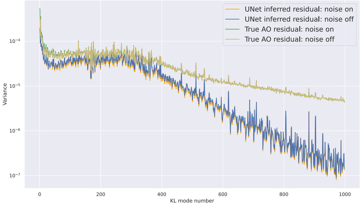
Figure 5: Variance (log) between KL modal weights of the inferred wavefront estimates and simulated ground truth
