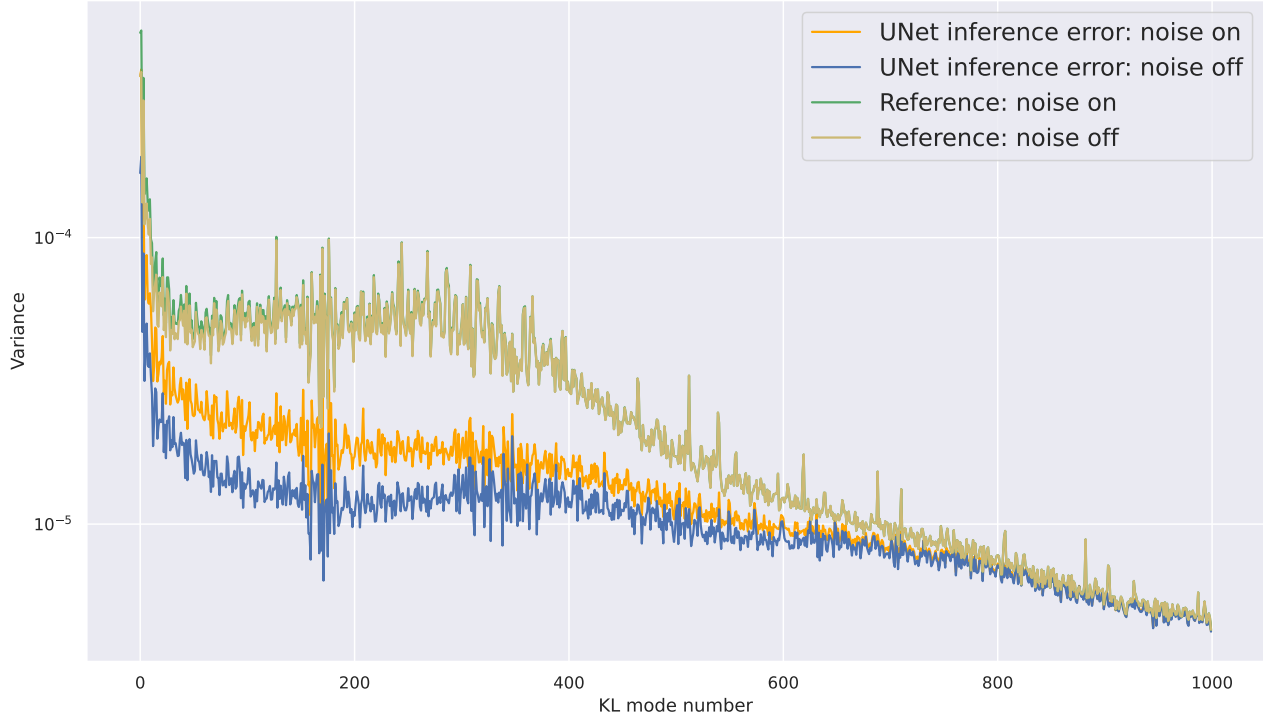
Figure 6: Variance (log) of the difference between KL modal weights of the inferred wavefront estimates and simulated ground truth
