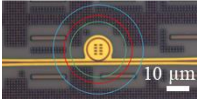
Figure 3: Optical top view of microring (purple and yellow) and etched cavities footprint to scale (green – 25 \mu\text{m} , red – 30 \mu\text{m} and blue – 40 \mu\text{m} )
