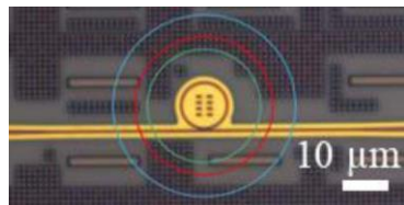
Fig. 6. Optical top view of microring (purple and yellow) and etched cavities footprint to scale (green – 25 μm, red – 30 μm and blue – 40 μm)
