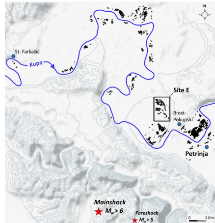
Figure 1. Map of sand ejecta and fissures along the Kupa river between Stari Farkašić and Petrinja (Baize et al., 2022).
