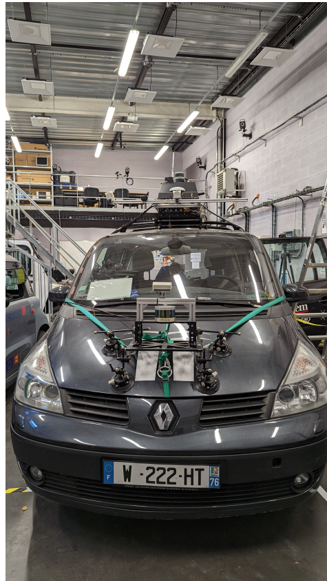
Figure 3. Intel RealSense camera mounted on the front of the vehicle.
