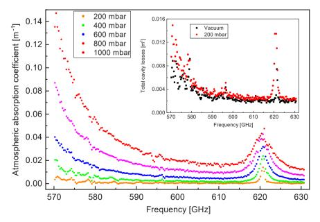
Fig. 8. Atmospheric losses measured using the cavity finesse for laboratory air at 22.5  $^{\circ}$ C, relative humidity from 48 to 53 %.
