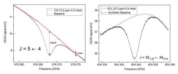
**Fig. 5.** Typical CEAS spectra covering approximately 20 MHz with a step size of 10 KHz. Left, a calibrated trace gas containing 73.2+/- 1.5 ppm of CO, acquisition time of 300 s. Right, 20.3+/- 0.4 ppm of SO<sub>2</sub>, total acquisition time of 600 s.
