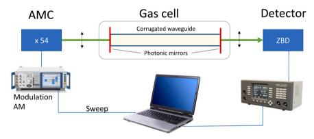
Fig. 2. Amplitude modulation characterisation of the cavity.
