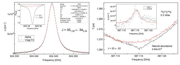
Fig. 7. Example spectra of CRDS. Left, SO<sub>2</sub> transition observed in an industrial gas sample at 0.38 mbar,  $5 \times 10^4$  ring-down events per measurement point, step size 100 kHz, total acquisition time of approximately 200 s. Right, weak absorption of  $^{18}O^{13}C^{34}S$  measured with  $10^5$  ring-down events per point, step size 100 kHz, total acquisition time of 300 s.
