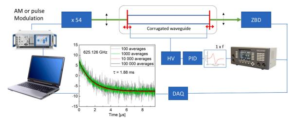
Fig. 6. CRDS configuration. Data acquisition is triggered at the end of the source pulse. Typical average ring-down signal are shown for acquisition lengths varying from  $100 \text{ to } 10^5 \text{ waveforms}$ .
