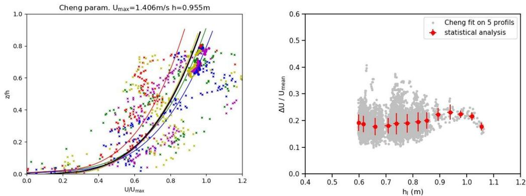
**Figure 7. (left) Examples of 5 successive profiles (5 minutes apart) of scaled velocities fitting by a Cheng's law on each profile (coloured curves) or on the whole data (black curve). (right) Evolution of the characteristic deviation from velocity data to the adjustment (Cheng's law on 5 successive profiles) as a function of the water level for the month of March 2019 (all values, mean and standard deviation).**
