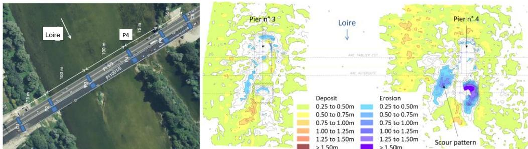
**Figure 2. A71 motorway double viaduct in Orléans (France) over Loire river: (left) aerial view of the bridge and (right) bathymetric surveys comparison between January 2018 and May 2016 (Chevalier et al. 2021).**
