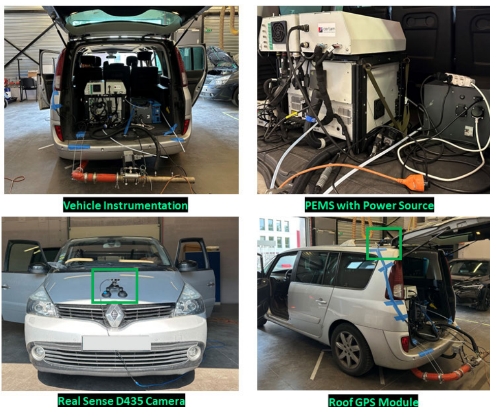
FIGURE 2. Instrumented vehicle for VAD construction.
