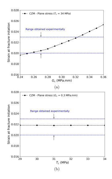
Figure 14: Macroscopic strain at crack initiation obtained using CZM (a) with respect to the critical energy release rate  $G_c$  for critical stress  $T_c = 34$  MPa and (b) according to the critical stress  $T_c$  value for  $G_c = 0.30$  MPa.mm. The blue dashed lines indicate the range of experimental uncertainty defined by mean value and standard deviation.
