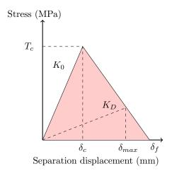
Figure 5: Illustrations of the cohesive traction-separation law.
