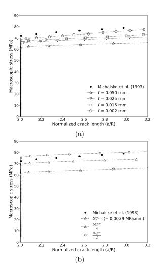
Figure 7: Phase-field fracture modeling of DCDC test [2]. (a) Impact of regularization parameter  $\ell$  for material constant  $G_c$  [2]. (b) Impact of  $G_c$  for constant regularization parameter  $\ell = 0.05$  mm.
