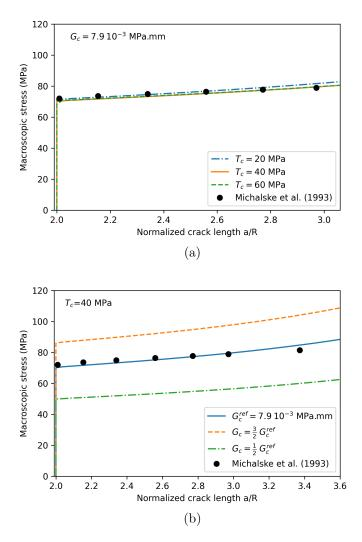
Figure 8: Impact of CZM parameters  $T_c$  (a) and  $G_c$  (b) on the quasi-static crack propagation for the linear elastic experimental case [2].
