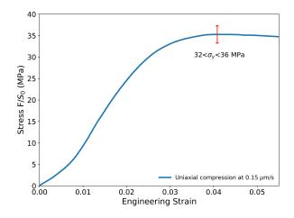
Figure 2: Monotonic uniaxial compression stress with respect to the compression strain applied at a constant crosshead speed of 0.15  $\mu$ m/s measured on a solid cylinder sample.
