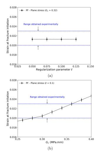
Figure 10: Macroscopic strain at damage initiation obtained using phase-field method (a) Impact of the regularization parameter  $\ell$  at constant  $G_c = 0.32$  MPa.mm and (b) dependence to the critical energy release rate  $G_c$  for  $\ell = 0.1$  mm. The blue dashed lines indicate the range of experimental uncertainty defined by mean value and standard deviation.
