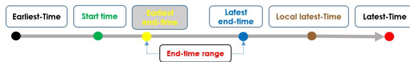
Figure 17. End-time range—global view: both end-time range bounds are located between the start-time and the latest-time.
