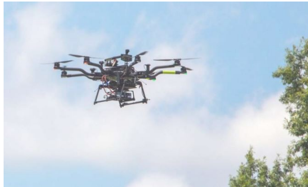
Figure 16: An Alta-8 small Unmanned Aircraft System testbed vehicle flies above NASA’s Langley Research Center in Hampton, Virginia. Flying beyond visual line of sight from observers on the ground required special approval from the Federal Aviation Administration and NASA. Credit: NASA / Bowman
