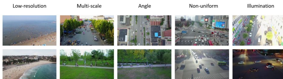
Figure 9: Challenges for aerial object detection: (i) low resolution, (ii) a wide range of scales, (iii) arbitrary viewing angles, (iv) non-uniformly distributed objects, and (v) varying illumination conditions. Images from the TinyPersons and VisDrone datasets. Adapted from [14]
