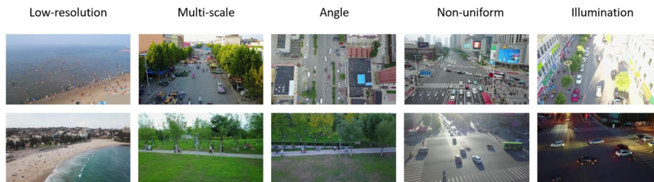
Figure 9: Challenges for aerial object detection: (i) low resolution, (ii) a wide range of scales, (iii) arbitrary viewing angles, (iv) non-uniformly distributed objects, and (v) varying illumination conditions. Images from the TinyPersons and VisDrone datasets. Adapted from [14]
