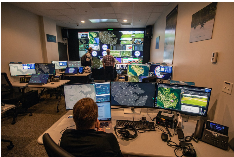
Figure 17: NASA researchers monitor the flight of an autonomous vehicle from the Remote Operations for Autonomous Missions UAS Operations Center at NASA’s Langley Research Center in Hampton, Virginia. The center facilitates “beyond visual line of sight” flight operations of small uncrewed aircraft system vehicles, also known as drones. Credit: NASA / David Bowman
