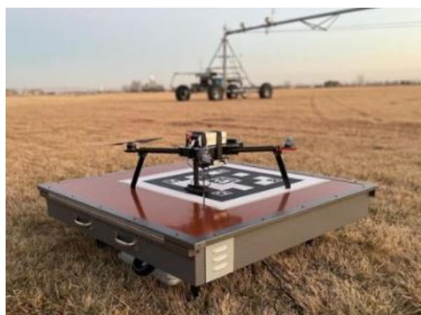
Figure 15: The WiBotic PowerPad Pro with an UAV landed on it [31].
