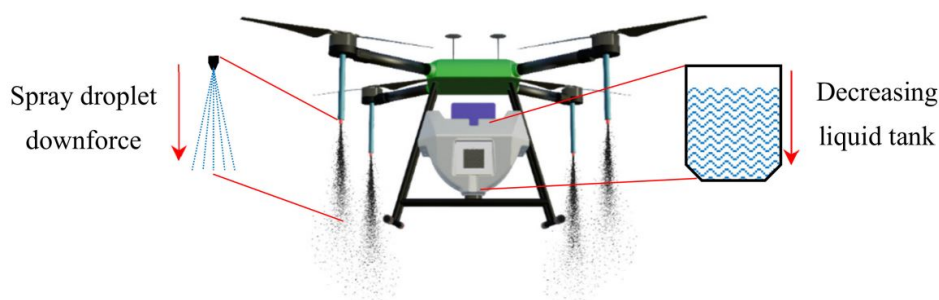
Figure 19: Autonomous sprayer UAV with key components highlighted: spray droplet downforce and the decreasing liquid tank level. Adapted from [40].
