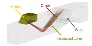
Fig. 2. UT inspection configuration, as it can be described with the CIVA software. the weld area joining two stainless steel plates is inspected using shear waves.
