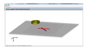
Fig. 1. ECT inspection configuration, as it can be described with the CIVA software. A stack of two aluminium sheets, affected by two narrow cracks, are inspected by a single coil.
