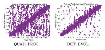
Fig. 6. Estimation of crack 2 opening (fourth parameter) in the ECT case when applying uncertainty propagation.
