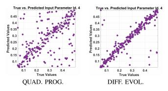
Fig. 4. Effect of additive white noise on the estimation of crack 2 opening (fourth parameter) in the ECT case. The signal to noise ratio is 20 dB.
