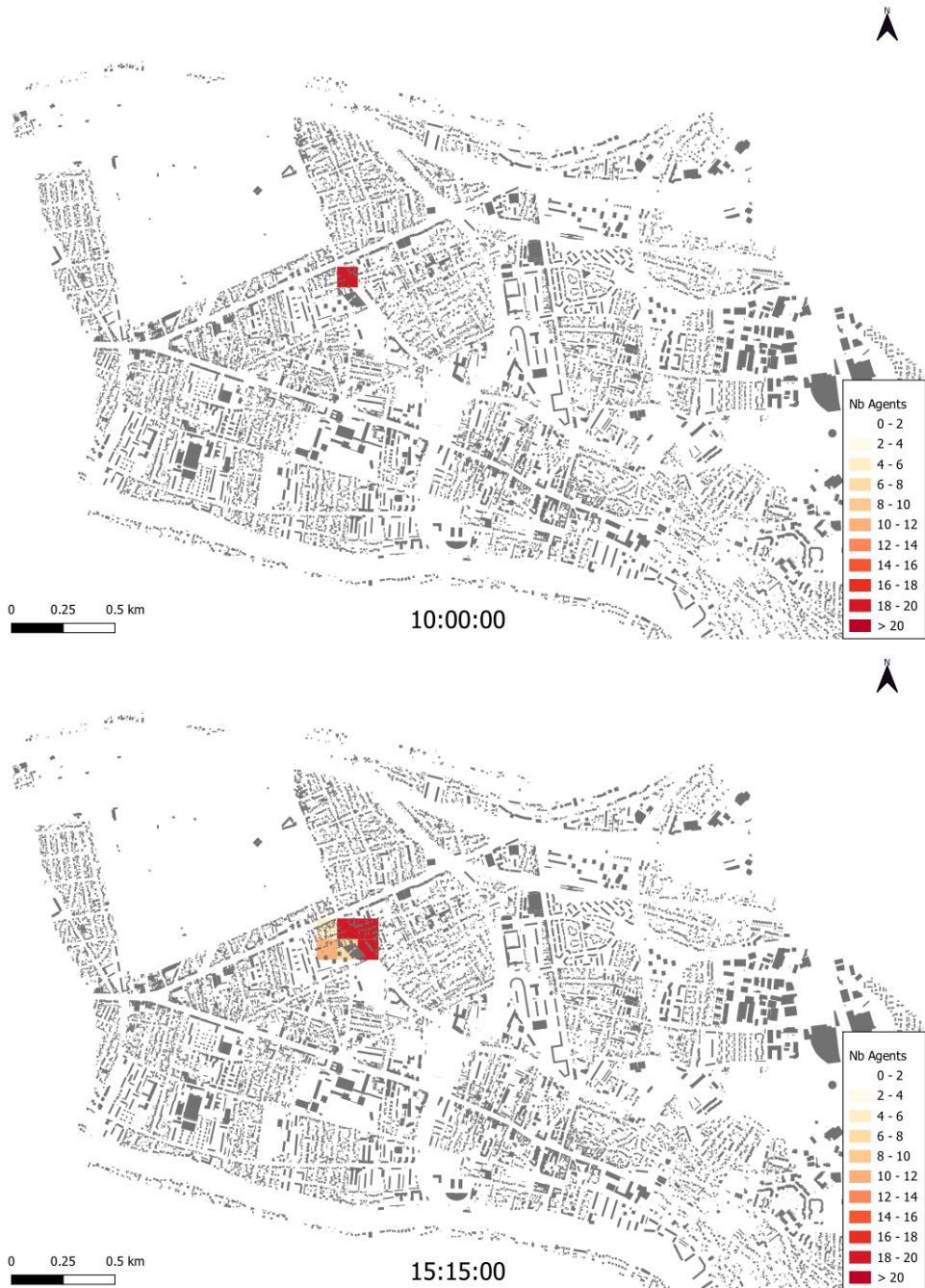
Figure 14: Difference in the number of individuals exposed to noise levels exceeding 65 dB(A) across 100x100 m. grid areas, during the quarter-hours starting at 10 a.m. and 3:15 p.m. respectively, comparing the configuration with the construction site to the one without it.
