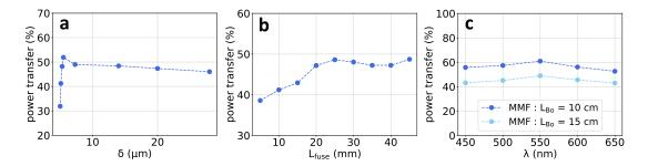
**Figure 6:** Measured power transfer of a hollow-core DCF coupler with a 300  $\mu$ m outer diameter hollow core DCF and a 500  $\mu$ m outer diameter BG MMF as a function of (a) the coupler length  $L_{fuse}$  and (b) the overlap parameter  $\delta$  between both fibers. (d) Measured power transfer after 15 cm (light blue dots) or 10 cm (dark blue dots) of propagation inside the BG MMF after the coupler.
