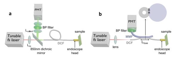
**Figure 1:** Typical nonlinear endoscopy scheme setup based on a hollow core DCF. Excitation and collected signal, respectively guided through the hollow core and the silica clad, are separated either with (a) a dichroic mirror or (b) a double-clad fiber coupler.
