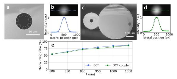
**Figure 7:** SEM of (a) the 7 capillary hollow core DCF and (c) the hollow core DCF coupler fabricated with it and a 500 µm outer diameter BG MMF. Imaged hollow core FM of the hollow core DCF (b) before and (d) after fabrication of the coupler, with a profile plot along the marked horizontal dashed line and a Gaussian fit (gray solid line). (e) Hollow core fundamental mode coupling ratio of the hollow core DCF before (blue dots) and after (green dots) fabrication of the coupler.
