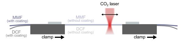
**Figure 3:** DCF coupler fabrication setup. Fibers, stripped of their coating, are clamped against each other and fused using a  $CO_2$  laser.
