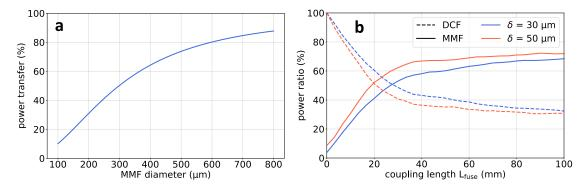
**Figure 2:** (a) Power transfer from a hollow core DCF to a MMF as a function of MMF diameter for a 300  $\mu$ m outer diameter hollow core DCF, calculated using Eq. 1 [18]. (b) Numerical simulations of the power distribution inside the hollow core DCF (dashed lines) and MMF (solid lines) as a function of coupling length, for overlap parameter values of  $\delta = 30~\mu$ m (blue lines) and  $\delta = 50~\mu$ m (red lines).
