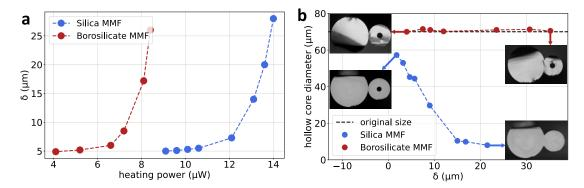
**Figure 4:** (a) Measured overlap parameter  $\delta$  between the DCF and the MMF as a function of the  $CO_2$  laser heating power, using a pure silica MMF (blue dots) and a BG MMF (red dots). (b) Measured capillary inner diameter as a function of the overlap between the fibers using a pure silica MMF (blue dots) and a BG MMF (red dots). The horizontal black dashed line depicts the initial inner diameter of the capillary fiber.
