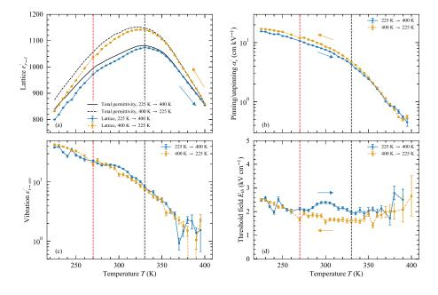
Figure 4. Relative permittivity for a measuring field of  $0.4\,\mathrm{kV\,cm^{-1}}$ , lattice contribution to the permittivity (a), domain wall motion contributions to the permittivity (b,c) and threshold field (d) as a function of the temperature.
