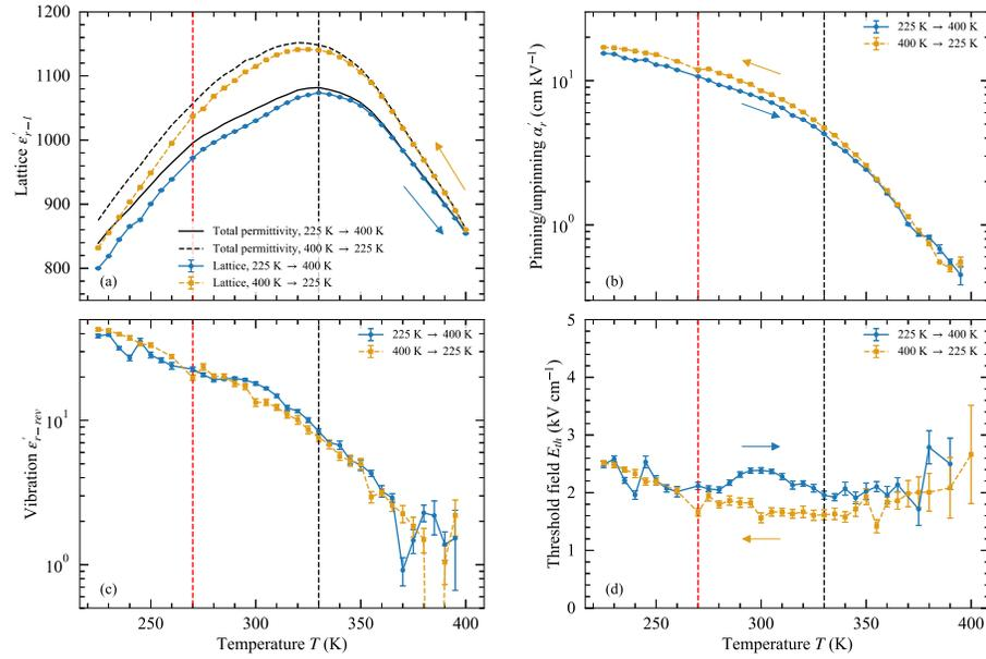
Figure 4. Relative permittivity for a measuring field of  $0.4 \text{ kV cm}^{-1}$ , lattice contribution to the permittivity (a), domain wall motion contributions to the permittivity (b,c) and threshold field (d) as a function of the temperature.
