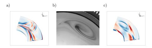
Figure 1: (a) Axial vorticity computed at Re = 95, with free surface condition. (b) Experimental visualization at  $Re \sim 30$ . (c) Axial vorticity computed at Re = 53, with frozen surface condition
