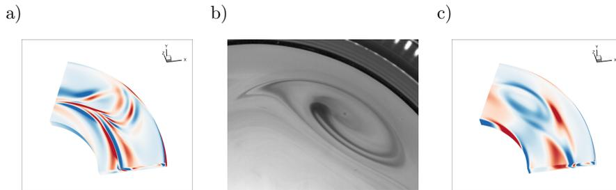
Figure 1: (a) Axial vorticity computed at  $Re = 95$ , with free surface condition. (b) Experimental visualization at  $Re \sim 30$ . (c) Axial vorticity computed at  $Re = 53$ , with frozen surface condition
