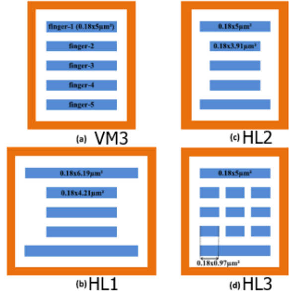
Fig. 8: Finger layout of the test structures. The DTI is shown in orange, whereas the five drawn emitter windows are colored in blue. [Esp16]. The emitter surfaces are: HL1 / VM3= 4.5 \mu\text{m}^2 , HL2 / HL3= 3.38 \mu\text{m}^2
