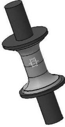
Figure 2: 3D view of the specimen and its steel mounting fixtures
