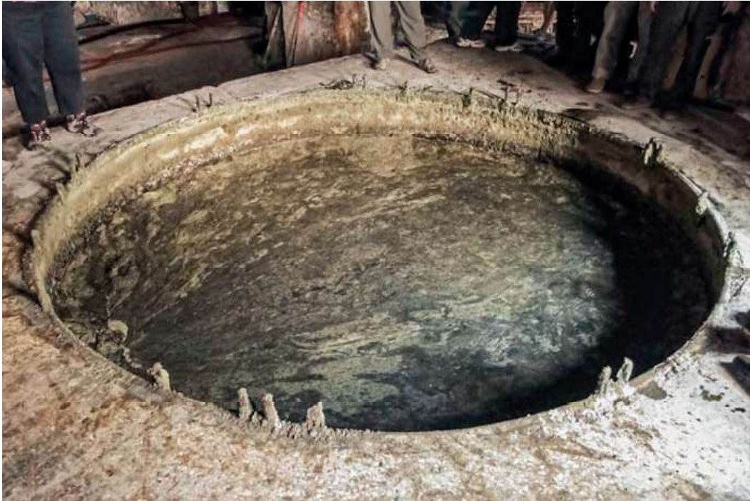
Fig. 1. Vat of Aleppo soap at the Al-Jebeili factory, Aleppo, Syria, 2010. Masses of saponified fat in process of formation – maybe the “piece of brine” floating on the surface, are visible in the foreground.
