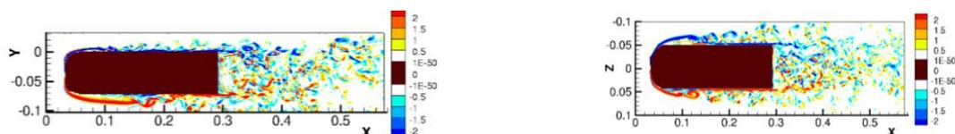
Figure 2: Unsteady flow for a slip condition: (left) spanwise component of the vorticity  $\omega_z$  in a vertical mid-plane ( $xy$ ) and (right) vertical component of the vorticity  $\omega_y$  in a horizontal plane ( $zx$ ) at mid-height of the body.
