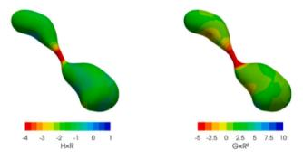
**Fig. 3.** Dimensionless mean (left) and Gaussian (right) local curvature of the droplet given in Fig. 4 at time  $t = 45.91 t_c$ . A video with the temporal evolution of this Figure is given in the additional material.
