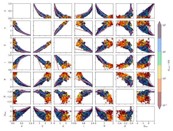
Fig. A.9. Scatter plot of shape parameters. Color by time remaining before break. The lines represent the case of oblate (solid red) and prolate (dashed blue) spheroids. The first column correspond to Fig. 6 in the manuscript.
