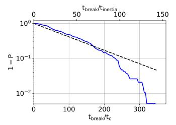
Fig. C.12. Survival probability for a given time  $t_{break}$ . Black dashed line corresponds to the constant breakup rate,  $\exp(-t\kappa)$  with  $\kappa = 0.021/t_{inertia}$ .
