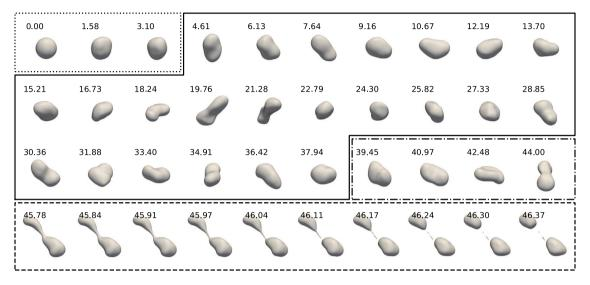
Fig. 4. Temporal evolution of a droplet interface. Time is given dimensionless  $(t/t_c)$ . Initial deformation (dotted line), oscillatory regime (solid line), no-return deformation (dash-dotted line) and capillary driven breakup (dashed line, the time between two snapshots is reduced). The corresponding video is included in the additional material.
