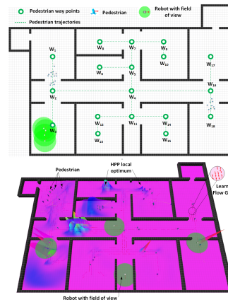
Fig. 5: Museum Scenario (Artificial Scenario). On the top, the scenario map and the set of way points following by 2 pedestrian groups. On the bottom, the scenario played with 4 robots following Hamiltonian path, flow grid learning and HPP computation
