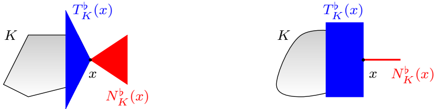
Figure 2.2: Illustration of the adjacent cone (blue) and normal cone (red) taken at some point on the boundary of a nonsmooth (left) or smooth (right) convex body.
