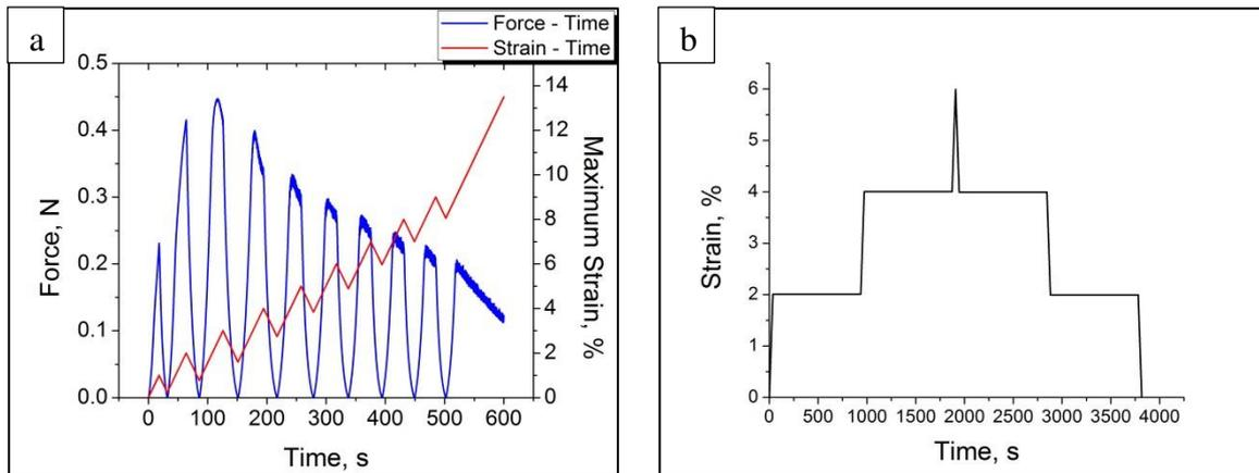
Figure 2. Loading profile for (a) cyclic loading test and (b) cyclic-relaxation test.
