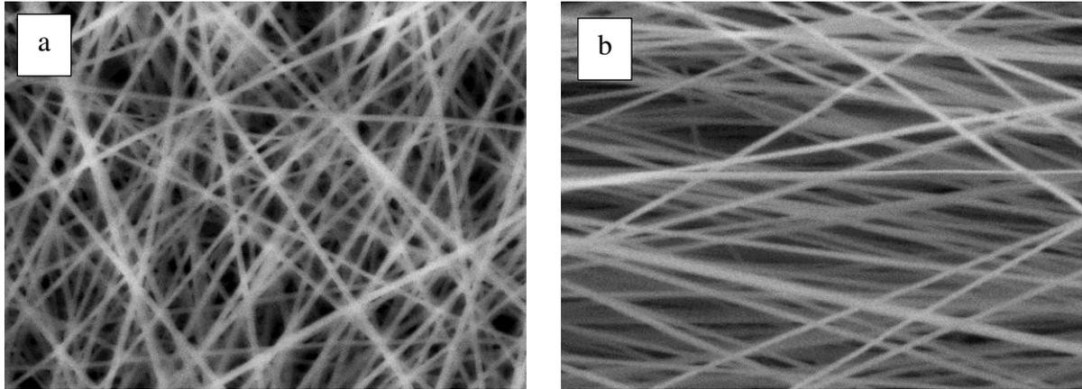
17 *Figure 16.* SEM images of nanofibrous membrane (a) before being stretched and (b) after
