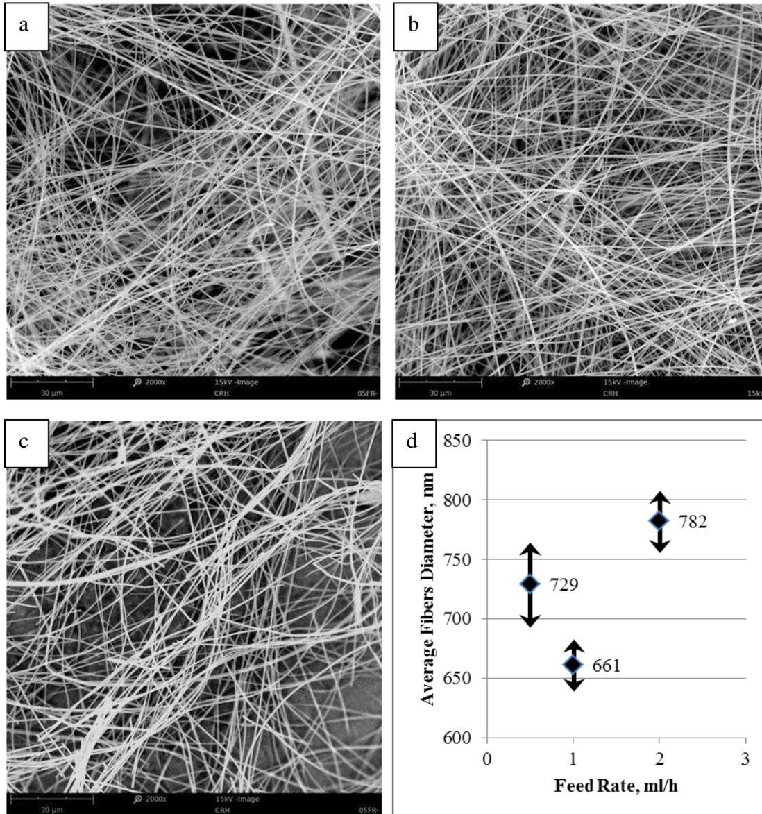
Figure 7. SEM images of Sample (a) F1, (b) F2, (c) F3 and (d) graph of average fiber diameter against feed rate.
