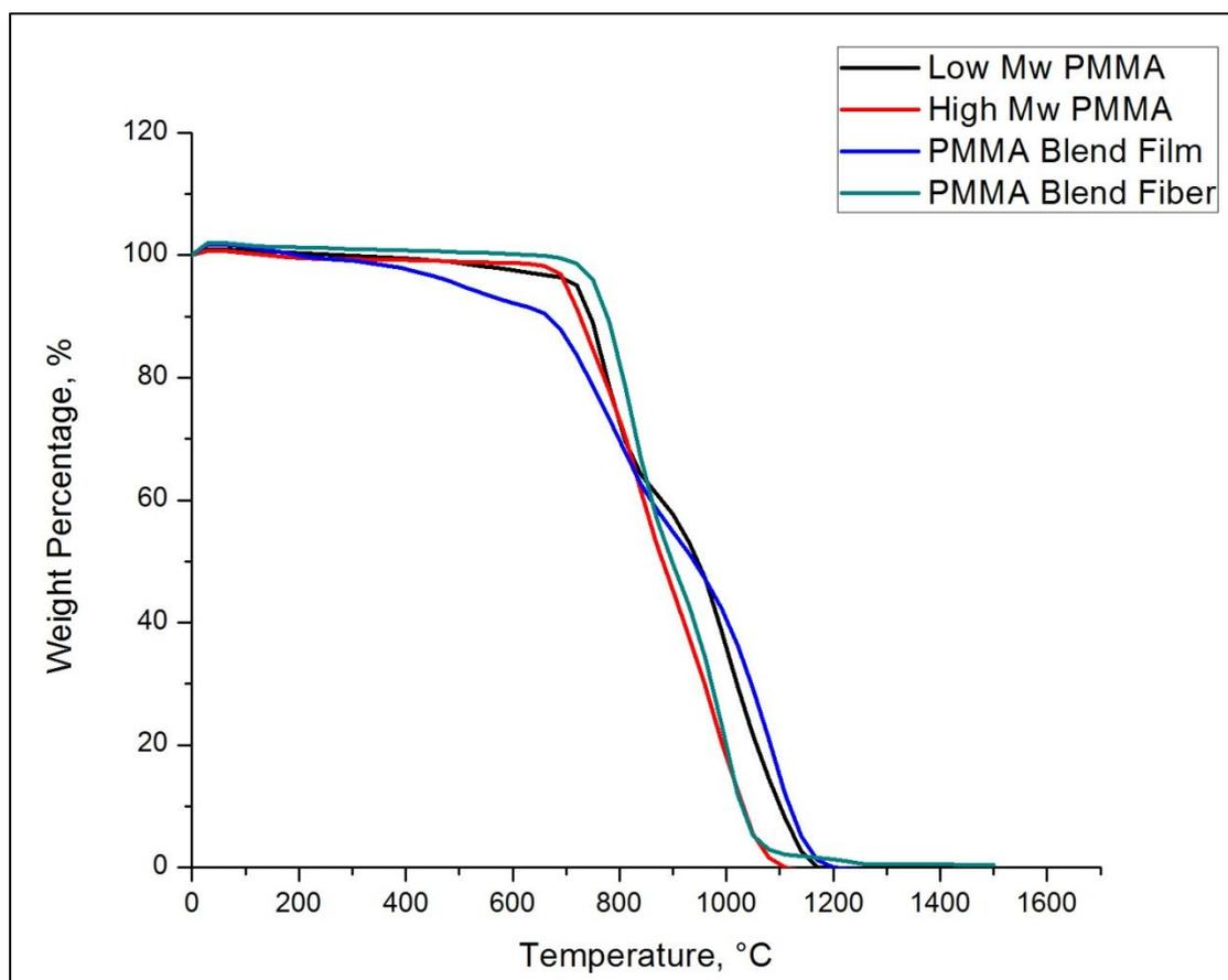
Figure 11. Graph of weight percentage against temperature obtained from TGA.
