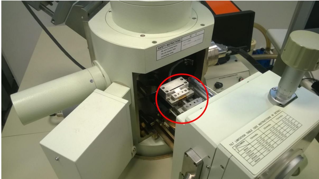
Figure 3. Red circle indicates the Deben tensile machine which is attached in SEM for in-situ tensile test.
