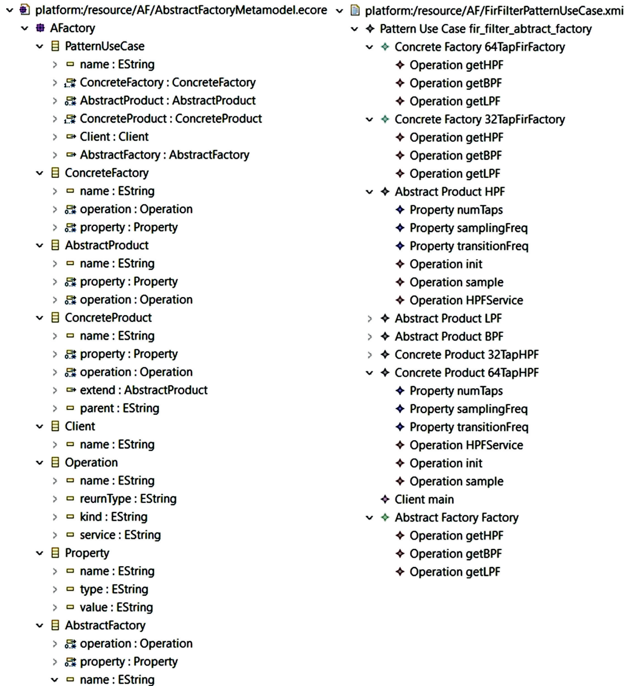
FIGURE 29: Abstract factory metamodel (left) and instantiated FIR filter model (right).
