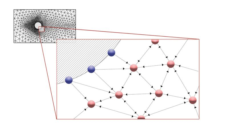
The training process has been performed on 3 differently refined meshes, depending on the Reynolds numbers, to ensure the mesh independence of the NN model. The loss function to be minimized during the training process is as follow:
