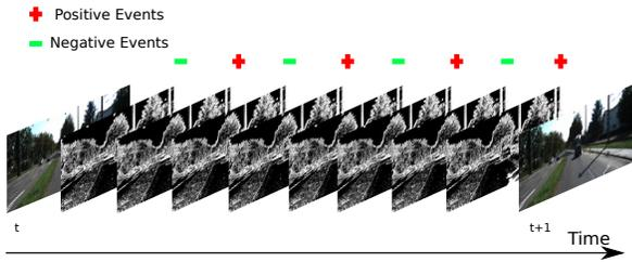
Fig. 3. Visualization of our event encoding representation.
