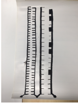
Fig. 5. A prototyped interface with syncopation patterns drawn onto paper with conductive paint, aiming to facilitate the experiential quality of rhythm.
