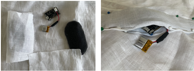
Fig. 3. The initial design of the sounding scarf included a pouch to embed the wireless IMU for movement sonification.
