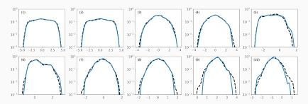
Probability density function of the amplitude of each mode over a trajectory of  $\approx$  1000 seconds. The CD-ROM results are presented in blue while the DNS is in black.
