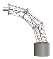
**Fig. 2** Robot manipulator using a stack of the proposed spatial mechanism.
