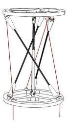
Fig. 16: Two potential design solutions for achieving a full orientation in  $\alpha$  and  $\beta$  accomplishing the condition of tensegrity ( $\{f_{c1}, f_{c2}, f_{c3}\} > 0$ ).
