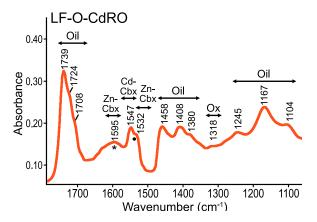
**Fig. 6.** FT-IR spectra of LF-O-CdRO highlighting the band in relation to the oil binder, the presence of amorphous (∗) and crystal (•) forms of Zn carboxylates (Zn-Cbx), Cd carboxylates (Cd-Cbx) and oxalates (Ox).
