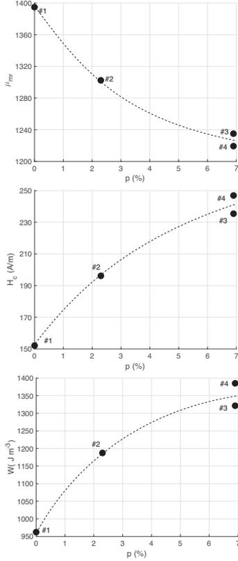
Figure 7: Maximal relative permeability (a), coercive field at  $H_{max}=8000A/m$  (b) and static magnetic energy density losses at  $B=1.5T$  (c) as function of cumulative plastic strain.
