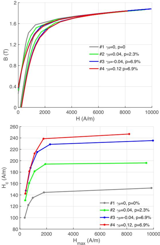
Figure 5: a) Experimental hysteresis cycles for the tested specimens. b) coercive field variation according to maximum magnetic field
