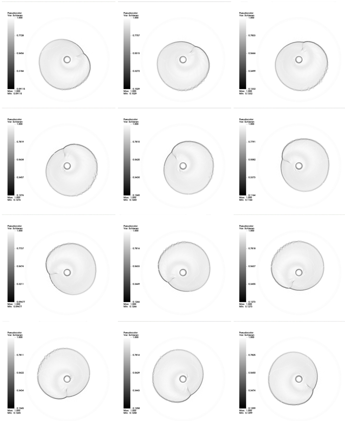
Figure 16: SWASI test on an unstructured quadrilateral mesh (261584 cells): Schlieren of the fluid depth ( h ) starting at t = 144.5 seconds and plot at time intervals of 0.5 seconds, top-left to bottom-right. The cusp rotates counter clockwise with a period of about 6 seconds.
