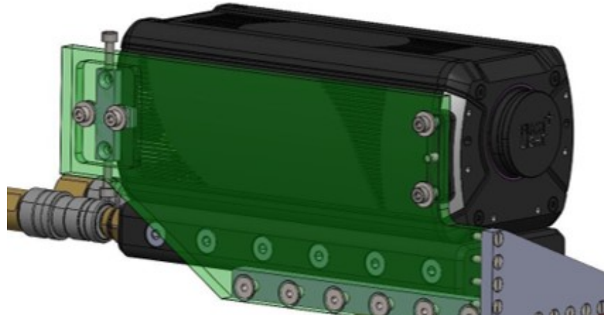
Figure 4. The tilt adjustment on the MLA plane is made possible by the two screws on the left
