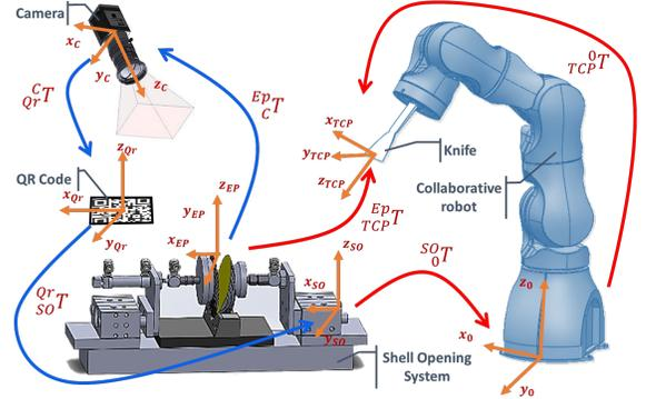
Fig. 8: Kinematic frames of cobot and vision systems
