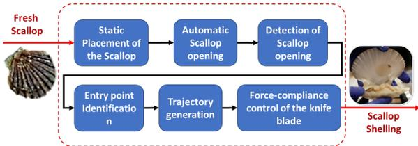
Fig. 2: System flowchart describing the process steps
