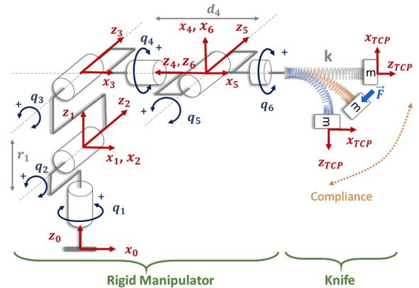
Fig. 9: CoboShell cobot kinematics chain.
