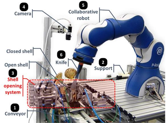
Fig. 3: CoboShell description : The shell is on a conveyor (1) in a vertical position on a support (2), the opening system (3) applies compliance to different types of valve surfaces using a vacuum system. The detection of the opening and the location of the entry point of the knife tip is achieved by a vision system (4). Finally, the adductor muscle is cut using a cobot (5) that guides the knife blade (6) along the flat shell for minimal material loss.
