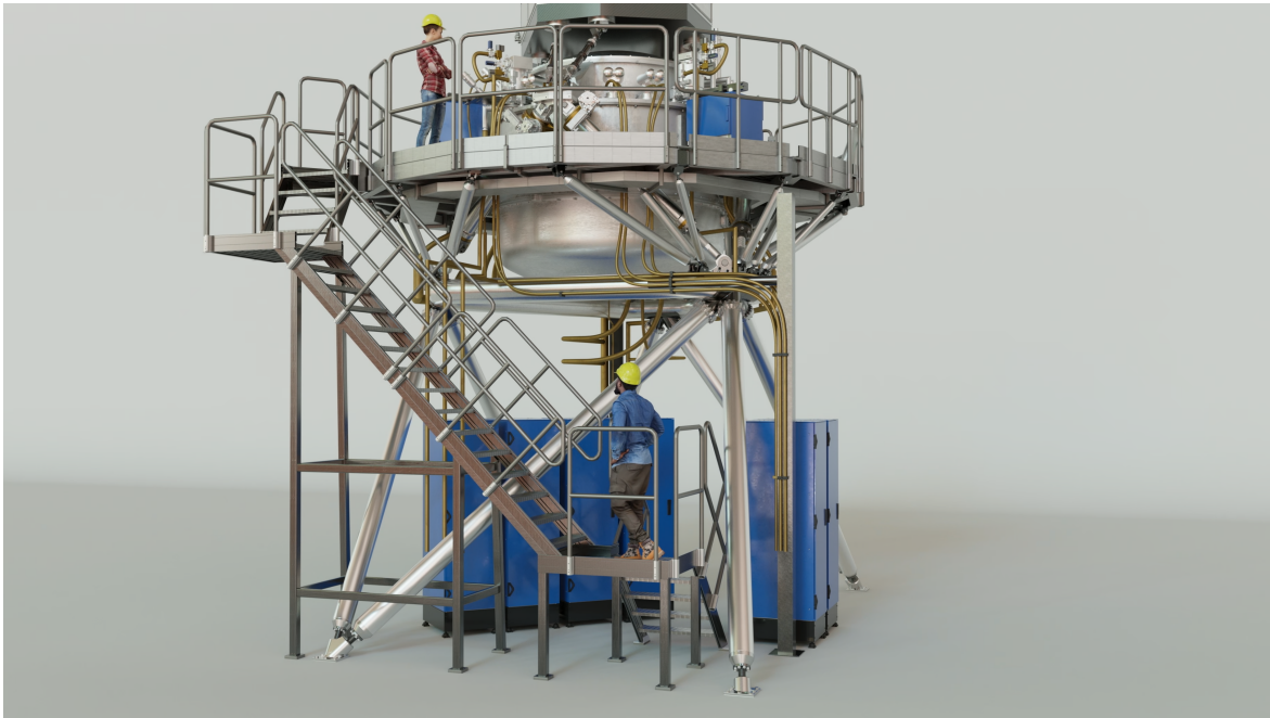
Figure 1. METIS will be located on one of the Nasmyth platforms of the ELT. At a height of 6m above the platform the light coming from the telescope enters the METIS cryostat, which hosts the entire optical path of the instrument down to the science detectors. It provides a very stable cryogenic environment, suppressing the thermal background emission. The SCAO wavefront sensor also resides within the cryostat. Rendering: ESO
