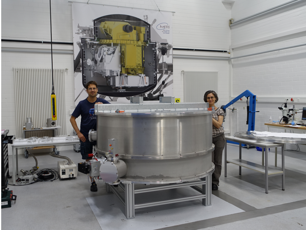
Figure 11. Test cryostat: A dedicated test cryostat is being set up for the tests of the SCAO Module. It will provide the operating environment of the SCAO module and allow for extensive testing before the integration into the METIS instrument.
