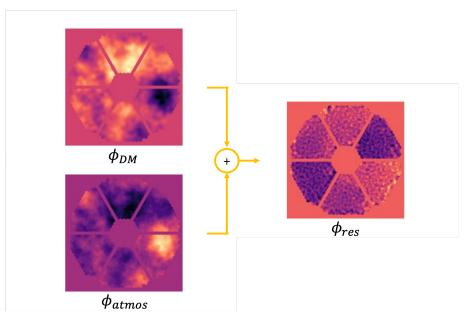
Figure 4. Example of atmospheric phase screen  $\phi_{atmos}$  and fragmented DM WF compensation  $\phi_{DM}$  that are summed and applied on the SLM as a single residual phase screen  $\phi_{res}$ . We note that this phase screen presents some differential pistons between each petal.
