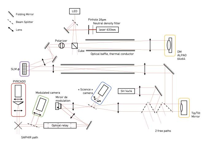
Figure 1. Optical path and components of the SESAME testbed.
