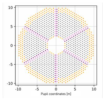
Figure 5. Actuator positions for a semi-ELT case with a pupil diameter of 20 m and an ELT-like inter-actuator pitch of  $d_{act} = 0.54 \ m$ . There are a total of 1218 actuators, that is 203 per fragment. Gray actuators are within the illuminated pupil while yellow actuators are the prolongation of the DM at the very edge or outside of the effective pupil. Pink and purple actuators denote the actuators situated along the spider arms.
