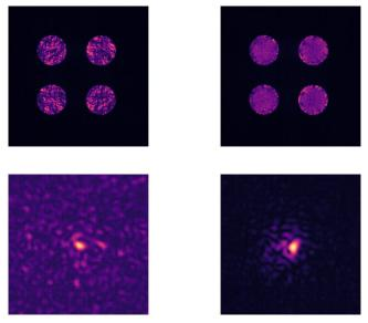
Figure 2. P-WFS and PSF images of **Left** open-loop and **Right** closed-loop AO system controlling 2000 modes of the ALPAO DM with a turbulence caracterized by  $d_{act}/r_0 = 1.2$ . The bright spot on the open-loop PSF image corresponds to a ghost reflection of the SLM.
