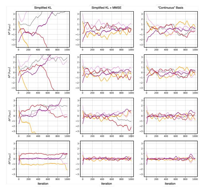
Figure 6. Differential piston fluctuations over 1000 iterations (2 s) for a P-WFS with 3  $\lambda/D$  modulation, based on the residual phase applied on the SLM. **Left** for a regular simplified KL basis, **Middle** when using the "MMSE" reconstruction, **Right** for the "continuous" basis. Each row refers to, from top to bottom, a Fried parameter of  $r_0 = 12, 15, 20, 30 \text{ cm}$  ( $\lambda = 500 \text{ nm}$ ).
